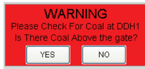
Figure 7: SCADA prompts for control room operator to check for inventory
